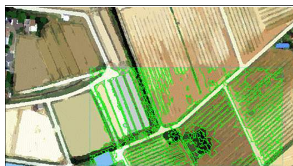
Figure 4: Example of applying the image segmentation and individual object extraction method to orthophoto image
